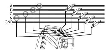
Fig. 1-3-1 Connection of Analyzer to 3-phase distribution system
