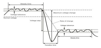
Fig. 3-3-4 Characteristics of a rapid voltage change
