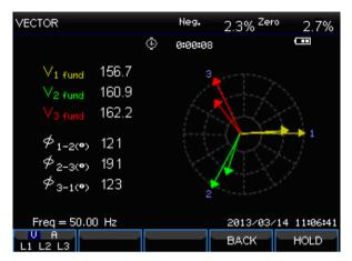
Fig. 2-5-1 Vector diagram for correctly connected Analyzer
