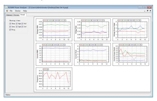
(3) Open log file with .csv format, user can directly open EXCEL file under windows or open it using this software. Click Y zoom button and then click data table, scroll up or down the mouse wheel to realize the zooming of Y-axis only. Click X zoom button and then data table, scroll up or down the mouse wheel to realize the zooming of X-axis only. Hold the mouse left clicking to make the left or right shifting of data waveform.
