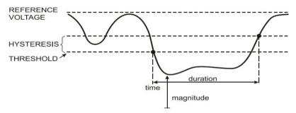
Fig.3-3-1 Characteristics of a voltage dip
