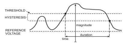
Fig. 3-3-2 Characteristics of a voltage swell
