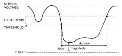
Fig. 3-3-3 Characteristics of a voltage interruption
