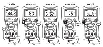
Note: Hz Input sensitivity varies automatically with voltage (current function alike) range selected. 1V range has the highest and the 1000V range has the lowest. Auto-ranging measurements normally set the most appropriate trigger level. You can also press the **RANGE** button momentarily to select another trigger level (Voltage range) manually. If the Hz reading becomes unstable, select higher voltage range to avoid electrical noise. If the reading shows zero, select lower voltage range.
